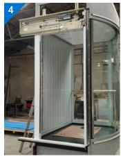
On approval of the 3D design, the bridal lift was factory preassembled in specific sections to fit the project schedule
