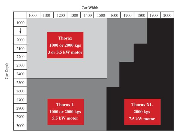
For a Thorax or Thorax L model, with a front open only car, for example, a car depth of 1500 mm will actually have a clear depth of 1450 mm, because of the rear wall. With an open through car, the clear car depth will be 1500 mm.
